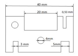
If the hook length fits within the 20 mm horizontal slot, then the maximum body thickness must fit in the 5 mm vertical slot.
